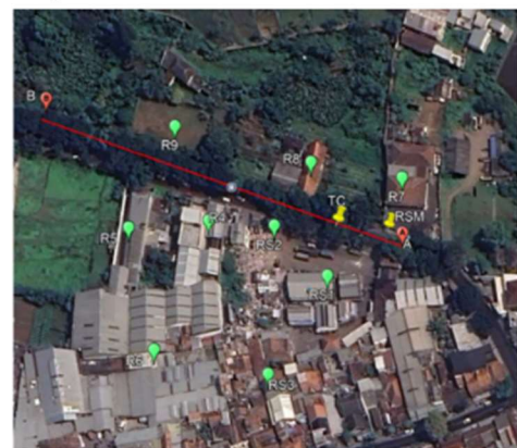
Figure 2. Spatial distribution of selected receptors and their relative positions along Sangkuriang Road used dor CALINE4 dispersion modeling
