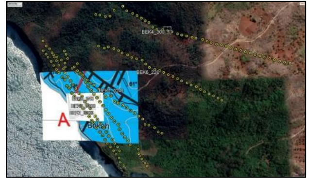
Figure 1. VLF-EM survey-line configuration in the Bekah karst area, Gunungkidul, showing six west–east measurement lines designed to intersect the dominant NE–SW structural trend.
