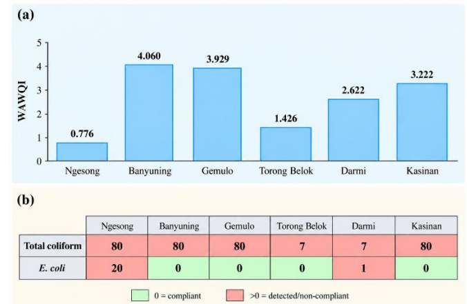
Figure 3. Comparison of (a) WAWQI values, and physicochemical classification, (b) microbiological contamination status of the investigated spring-water sources in Batu. All six springs fall in the excellent water-quality class. Microbiological contamination status in CFU/100 mL unit.
